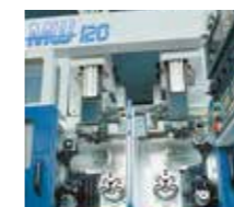
Machine Tools -Twin Spindle CNC Chucker -In-Line Opposed Twin Spindle CNC Turning Machine
