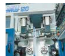
Machine Tools -Twin spindle CNC chucker -In-line opposed twin spindle CNC turning machine
