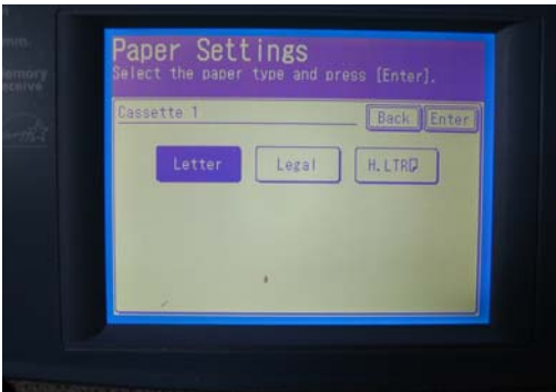
Users need to adjust the settings screen after supplying the device with legal size paper.
