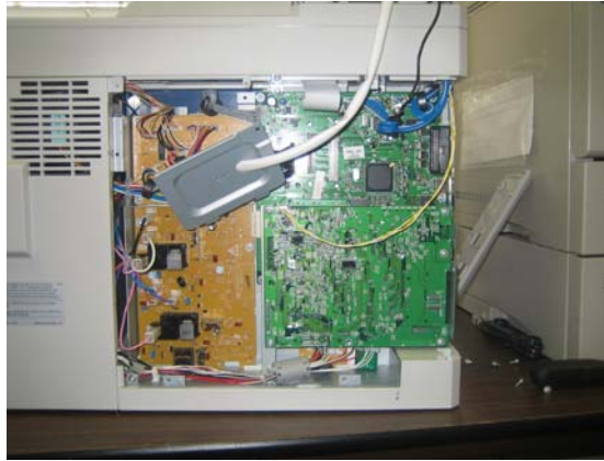
The motherboard can be accessed from the back of the F-560. A screwdriver is required to remove the metal cover.
