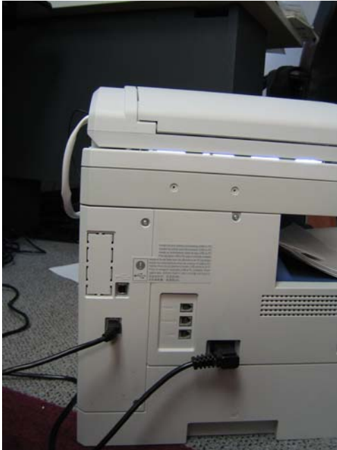
Connectors for USB, Ethernet, and fax can be found on the left side of the device.
