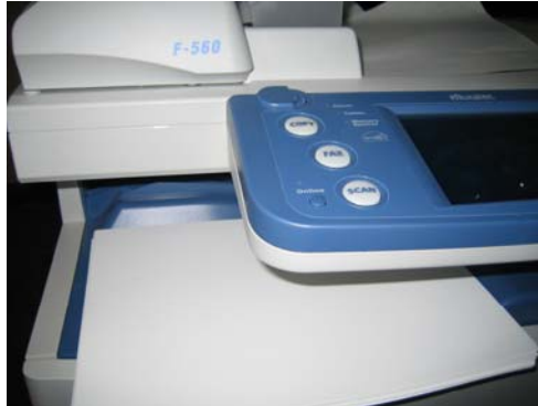
The 250-sheet output bin is found directly below the ADF.
