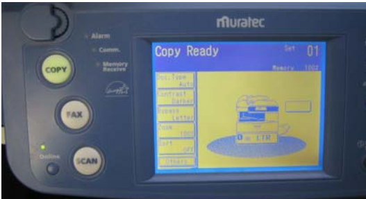
Copy controls are arrayed on the left side of the touch console. The "Others" button leads to a screen from which users can control duplexing, combine, and macro buttons.
